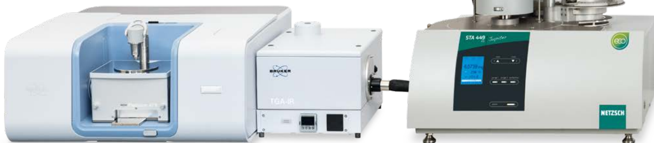
FT-IR Bruker Invenio ATR coupled to STA 449 F3 Jupiter® with automatic sample changer and QMS 403 Aëolos Quadrol
