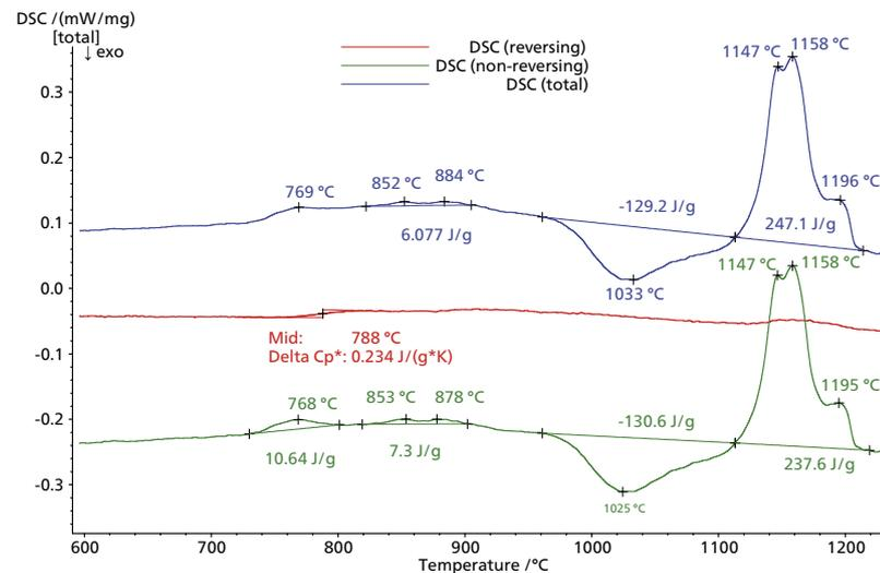
This TM-DSC measurement was carried out in a synthetic air atmosphere at a heating rate of 3 K/min and amplitude of 0.5 K/min for a period of 60 s. High-platinum crucibles with pierced lid were used. The sample mass amounted to 45 mg.
