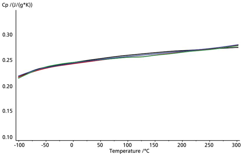
The specific heat capacity in the sub-ambient temperature range can be determined up to 300°C by means of the steel furnace (-150°C to 1000°C) and the DSC- $c_p$  sensor type E.
