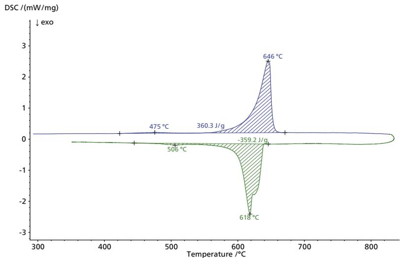
Pt crucibles with an  $\text{Al}_2\text{O}_3$  liner were used in order to prevent chemical reactions between the melt and the crucible material during a DSC measurement. Oxidation was avoided by using an argon atmosphere.
