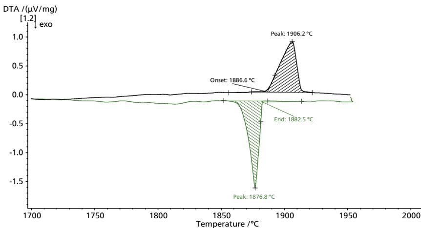
DTA measurement on vanadium in crucibles made of zirconium oxide (ZrO<sub>2</sub>); heating rate 20 K/min, cooling 75 K/min in a helium atmosphere.
