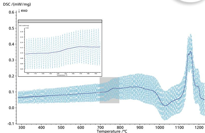
The simplest evaluation of a typical TM-DSC measurement is the determination of the total heat-flow curve as an average value of the modulated heat-flow differential curve. Modulated signal (light blue curve) and average values (dark blue curve: total heat flow).
