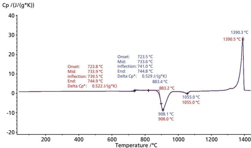
Excellent reproducibility and the detection of weak phase transitions (glass transition) can be achieved by simply combining the right furnace with the right sensor. These DSC runs were carried out with the Pt furnace and by using DSC- $c_p$  sensor type S.
