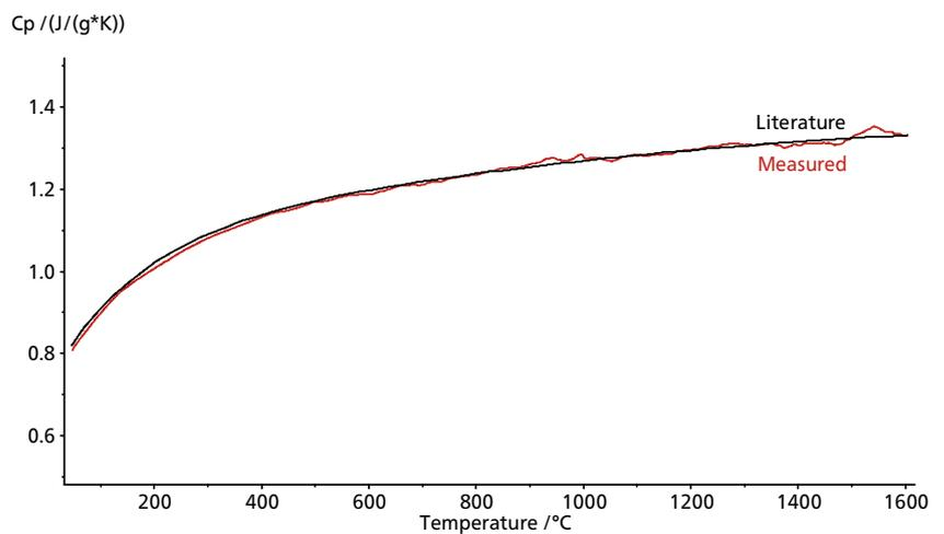
Highly accurate determination of the specific heat capacity across a wide temperature range. For these measurements, the rhodium furnace and the DSC- $c_p$  sensor type S were used.
