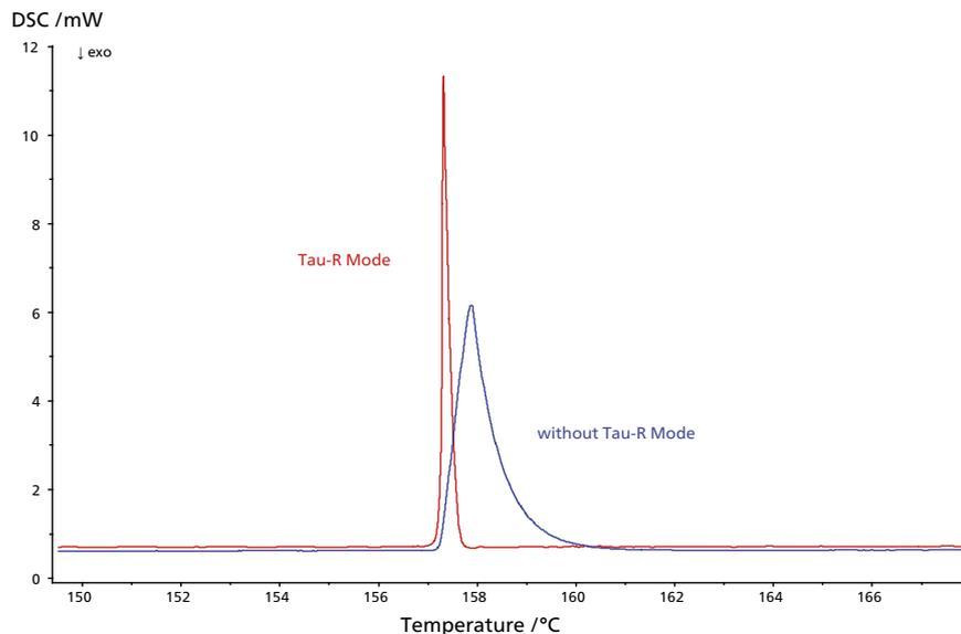
Correction of the thermal resistance and the time constant lead to defined peaks (*Tau-R*<sup>®</sup> Mode)
