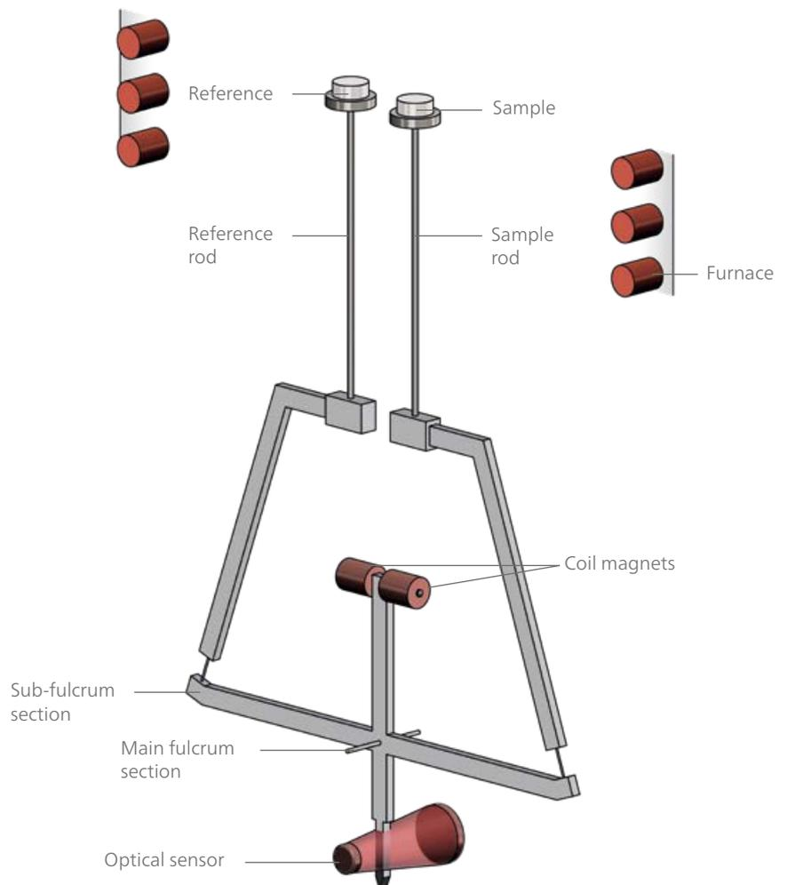
Schematic design of the top-loading differential balance of the STA 2500 *Regulus*
